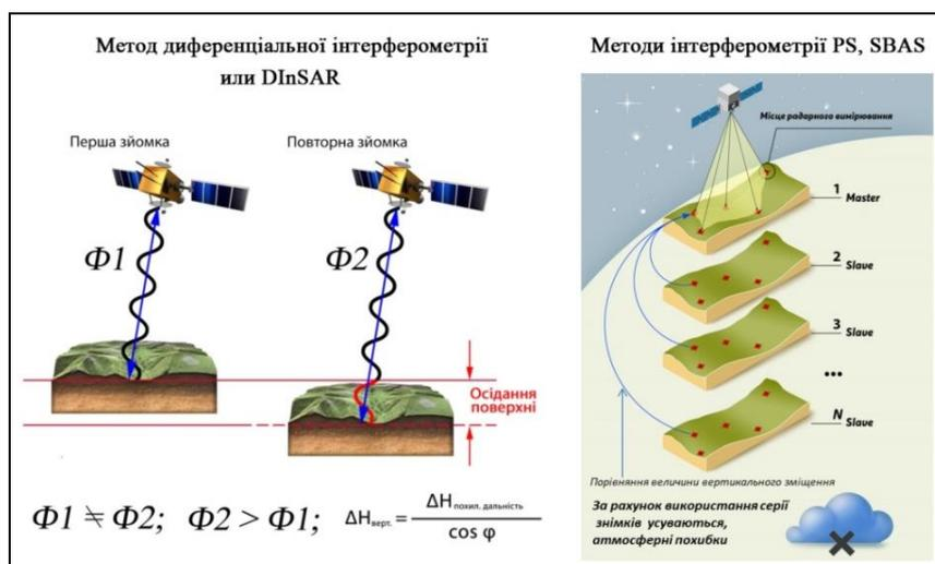
Figure 1 Schematic explanation of interferometric methods DInSAR, PS, SBAS
